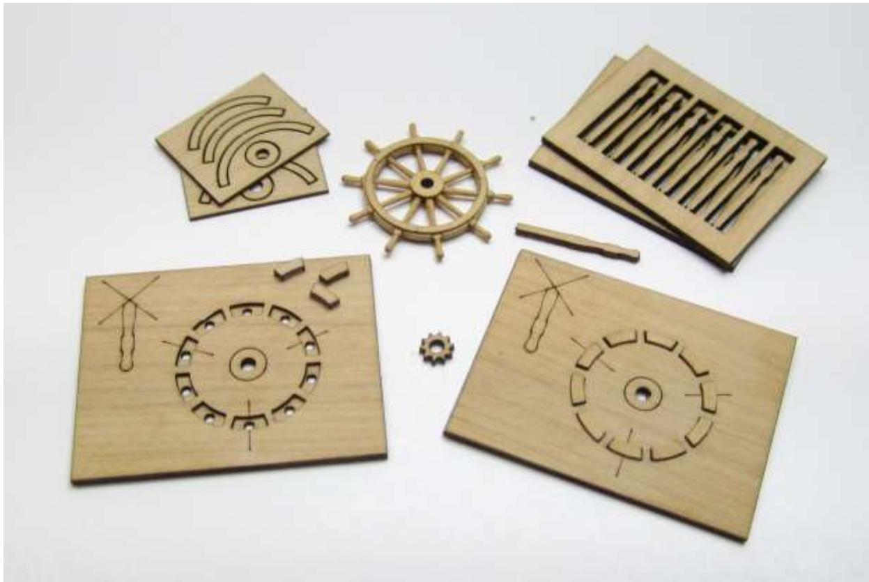
The first step would be too lightly sand both sides of all the sheets containing the pieces so you can remove the laser char before releasing them.
