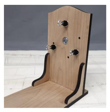
Lets turn our attention to the etched side of the head stock. Insert another small washer over each tube and then use the small tube clamps to secure each gear assembly. But once again, don't make these too tight at all. Make sure that the small gear will turn freely. Tighten the set screws on the tube clamps to secure them. See below.
