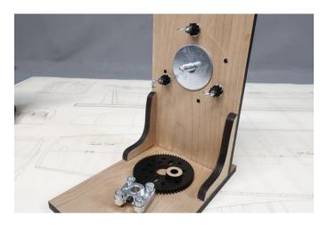
Also have the large gear at the ready along with the wooden washer/spacer. You can have the aluminum hub ready as well with the four set screws installed.
