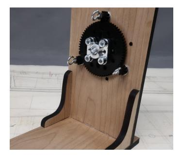
Lastly, place the hub in position so the four registration screws sit into the four holes on the gear. Tighten the set screw on the side of the hub. Just as before...not too tight. You want this gear to spin freely. That cant be emphasized enough.
