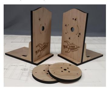
Sand the surfaces well and apply several coats of wipe on poly or other protective finish. To complete step one, take the two laser cut discs and insert the screw eyes into the laser cut pilot holes.
