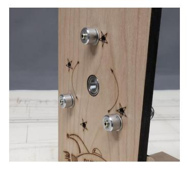
Next, use one large washer and a smaller ¼" washer while slipping the remaining machine screw through the bearing hole. Do this from the etched side of the head stock. See the photo on the top of the next column.
