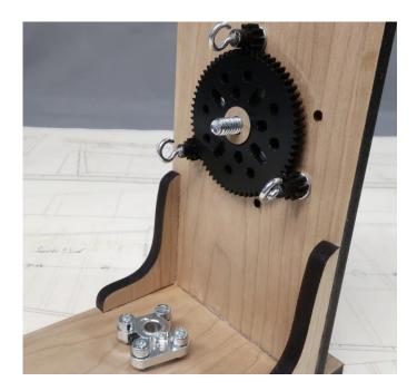
The last photo on the previous page shows the large gear in position. Note how the wooden spacer washer is pressed into the bore of the gear and inserted onto the machine screw. You may want to orient the small gears first so the open eye screws all face the same way. This isn't needed but can make tying the thread onto the hooks easier.
