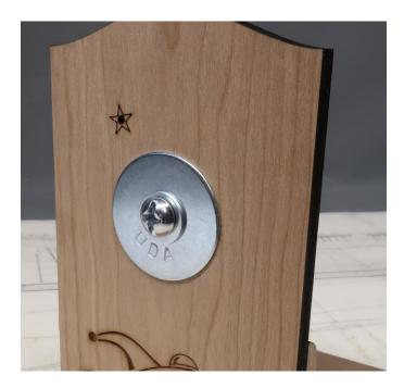
Turning your attention to the inside of the tail stock, place the remaining large washer over the machine screw. See below.
