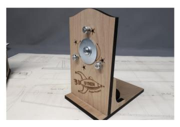
On the inside of the head stock, place the remaining large washer onto the machine screw. See photo below.
