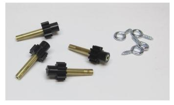
into each gear. Make sure you put the tube in the correct end of the gear. They will be so tight that it is impossible to remove if you screw up and insert it into the wrong end. You will need to gently hammer the tubes into the bore of each gear. Place the gear on a flat surface with the narrow end facing down on the
