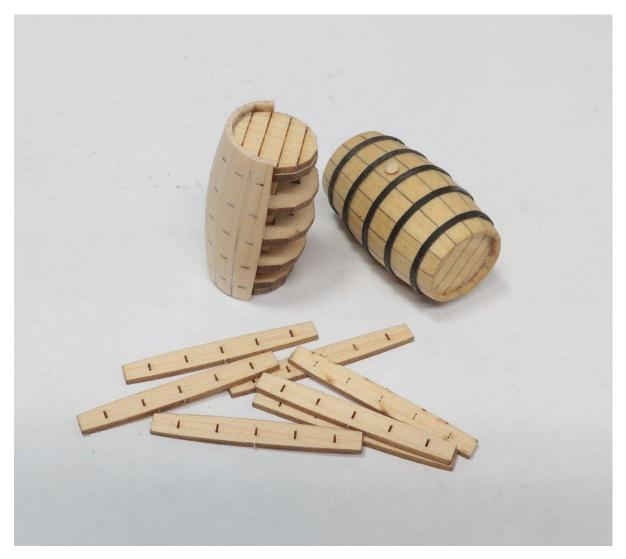
Use the etched line in the center of each stave to line it up properly on the barrel. It will line up with the center disc. Then just continue all around the barrel until all 14 staves are completed.
