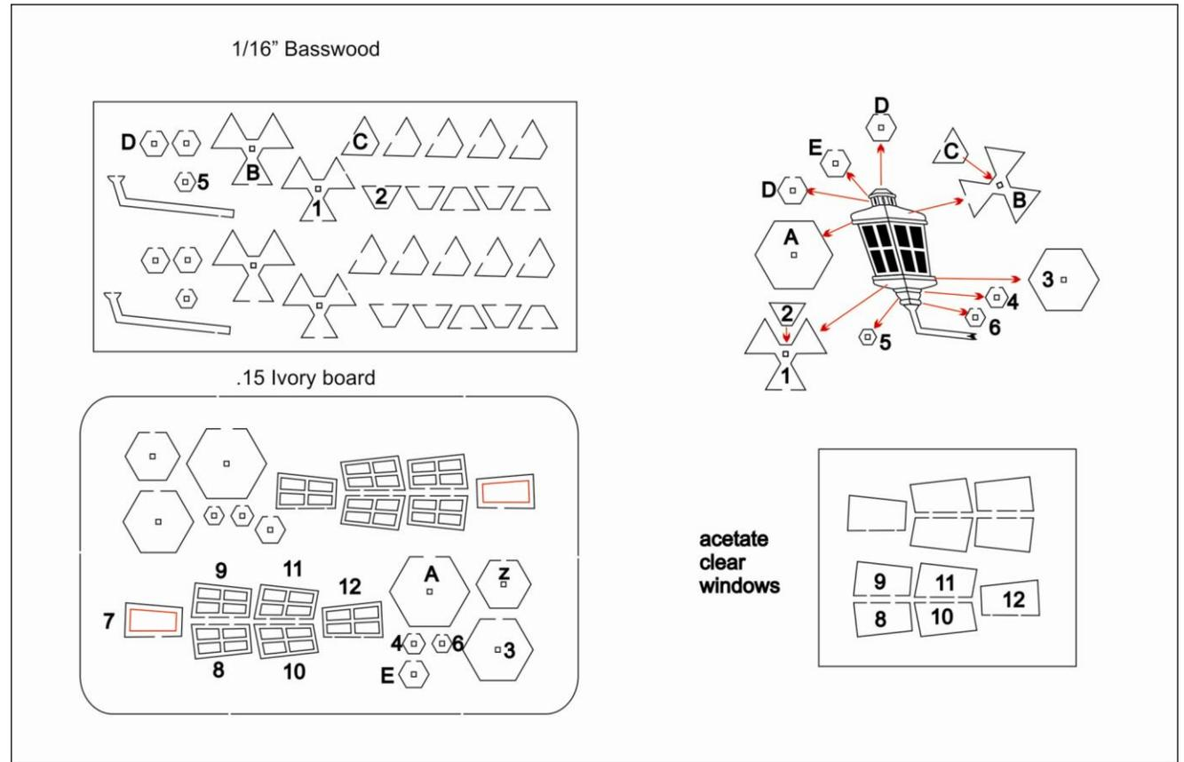
Remove part #1 from the laser cut basswood sheet. This piece looks like a "Y" shaped piece and will become the basis for creating the hexagonal bottom of the lantern. It is sometimes difficult to take a hexagon and sand it to shape consistently without altering the neat, clean hexagonal facets. To overcome this, you will be shaping three facets at a time.
