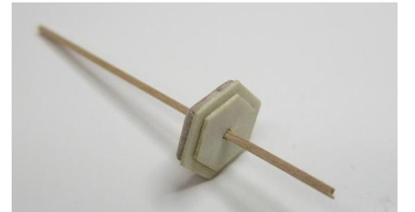
Remember, you must be able to remove the assembly from the stick so don't use too much glue. Slide it onto the stick with some space
