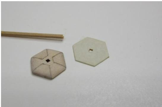
Remove part # 3 from the thin laser cut board. Also take the 1/32" x 1/32" boxwood strip provided with the kit. Very gently file the laser
