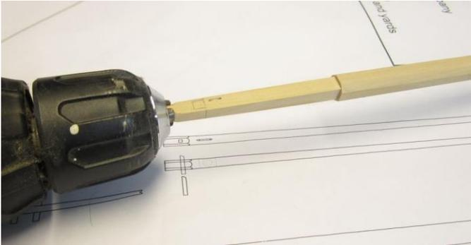
Then finally, I was able to finish up those sheaves so they looked good. To simulate the sheaves I used a #11 blade and some round needle files....you can use whatever you feel most comfortable with. Here are the final results below. This was done after I created the stepped portion or "shoulder" in the mast as you can see. The shoulder was just done by hand. The cedar worked very well for this operation and I was happy with the results.
