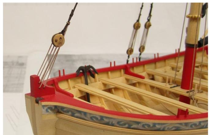
With these lines completed, you can start to re-tension them as needed. Then permanently glue them at their belaying points and add some rope coils.
