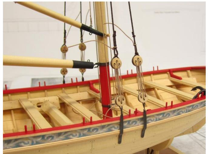
The lanyard run between the deadeyes is rigged using .018 light brown rope. This is done in the traditional way you are familiar with. Just try and keep the distance between deadeyes consistent.
