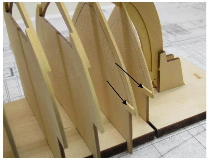
Then once this is finished you must test the frames in their slots on the build board. They will be very snug by design initially. You don't want these loose and falling out of the build board. But you don't want them too tight either. You want to be able to easily remove them
