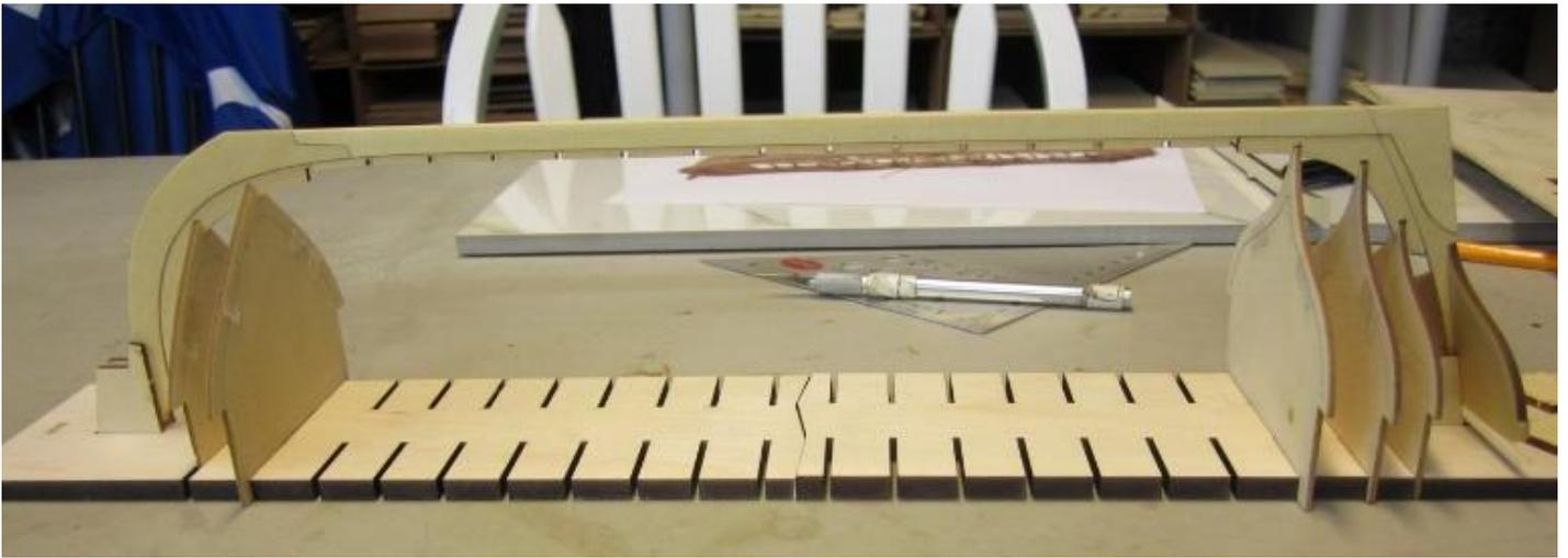
Above you can see what the keel assembly looks like after being tested on top of the five single part frames. Note how the two halves of the build board are not glued together. You should never glue the two halves together. Keep them separate for the time being. You can remove the keel assembly while you are building the two part frames next.
