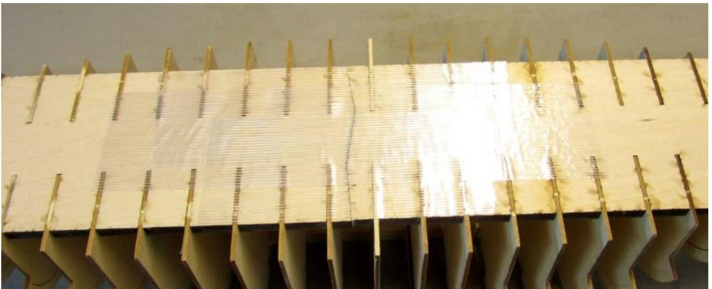
Here is the model after it was completely faired. You can use the laser char on the edge of each frame as a guide as you continue fairing as
