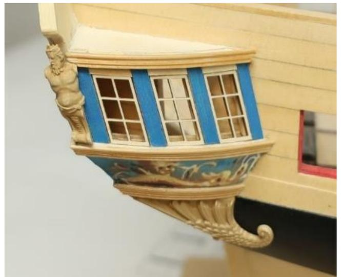
You will need to bend this to get it to lay against the surface properly. I also had to file out the aft edge of the molding so the figure would fit. I actually used a sharp miniature chisel after the molding was glued into position. I think you can
