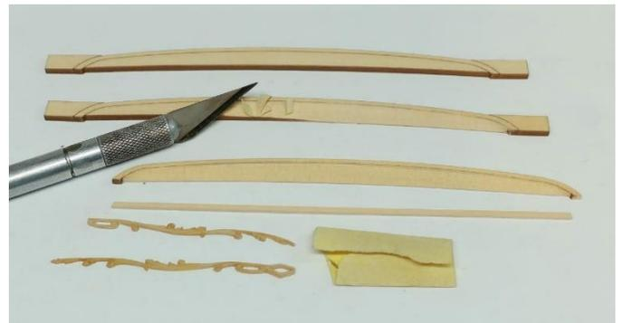
The photo above shows the cove in stages. The top shows the untouched example straight off the laser cutter. Notice the laser etched line to indicate the molding along the top edge. There are also some handles on either side which will eventually be removed. They are convenient for holding the cove while you shape it. In addition, along the bottom it is notched out so you can add a strip of wood which will become the molding along the bottom of the cove when you are done shaping it.
