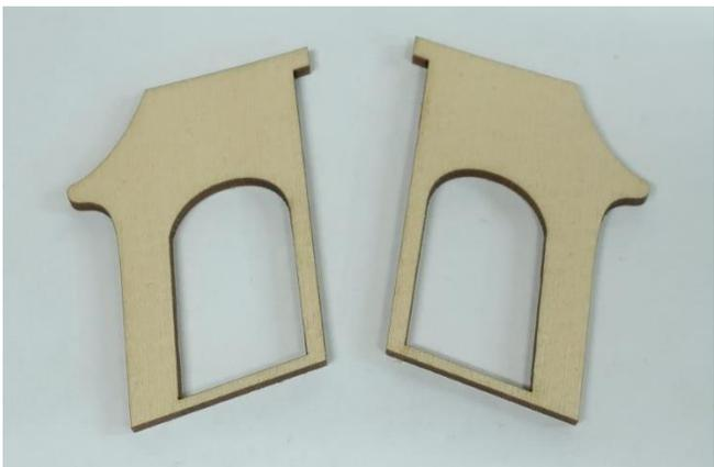
These are glued to the forward side of the transom where the quarter galleries will be. But it's not that simple. It never is right? As usual they are laser cut slightly over-sized. You must first bevel the side that sits against the hull planking. It will need some careful beveling. You also need to take enough material off of that side so it also leaves a consistent lip around the window on each side. Just like the other stern windows. This is so we can push those window
