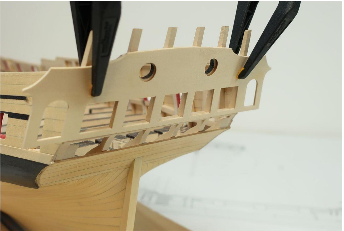
*View of the model with the transom clamped in position.*
