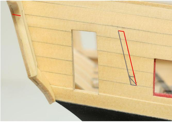
Well actually you will just have the forward pencil line. Shown in red. Then you need to add another line about  $\frac{3}{64}$ " aft of it. This represents the shell thickness of the gallery. Also note how I defined the  $\frac{1}{8}$ " frame at the bottom. This will be the first gallery timber we add to the model. That was the wide strip on the bottom of your paper template.
