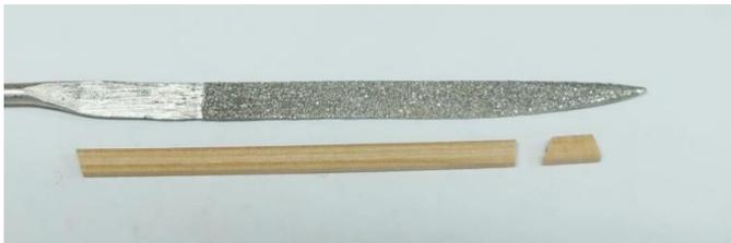
Then the fluted column was added between these two pieces to complete each column. These are laser cut from .025" thick boxwood. They have laser etched flutes. You may have to adjust the length or angles on each end for the best fit. They were cut a bit longer than needed.
