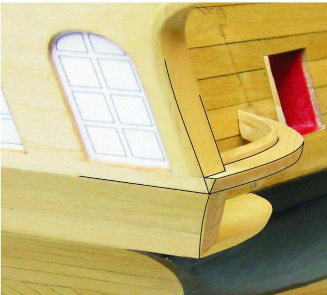
the bevels and fairing outboard. It is a complex beam. If you bought the laser cut pieces for this chapter you will find this beam on sheet "J".
