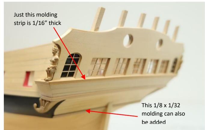
In the photo above you can also see that I tested the resin drop in position under the stool as well as the figure that sits on the end of the transom.
