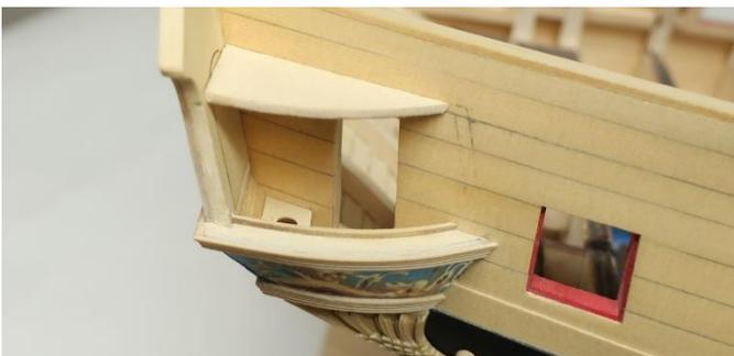
few spots of glue so they were just temporarily tacked in position. Then I placed a laser cut window temporarily so I knew where the next column would go. I marked the position in pencil. Do this carefully so all your windows fit. It's good to do a dry fit first of all the pieces. Use rubber cement to temporary hold the uprights in position while you tweak them for their best position. See below.
