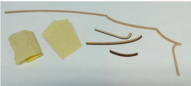
In the photo above, you can see the molding that is finished above a few pieces that weren't. I sanded off the laser char with some 320 grit sandpaper along the bottom half of each segment. By folding small pieces of sandpaper and cutting a curved sharp edge on the paper made it easier. It allowed me to clean up the face of the etched area. You will never get it all
