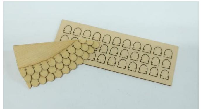
Note that the little etched lines in each shingles are not on your laser cut parts because that turned out to not be a good idea. They were added to give a reference for how much of an overlap on each row of shingles was needed. Just do your best to overlap each row so they look best and consistent.
