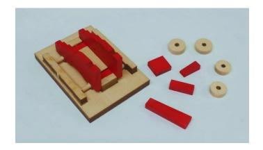
Next I added the two remaining wood parts on the front and back ends of the carriage. These parts are slightly longer so you have to sand them for a nice fit. Finally I also added a 1mm round bar across the center. It goes through the hole in the sides of the carriages...see below. You will need to buy some 1mm round brass rod.
