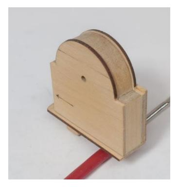
The same is true for the other side....Note how the first layer you put on is sanded flush with the edge of the core. AND the top is also sanded flush but the rounded section is left alone. Don't remove the char on that. You want the rounded hood to be perfectly shaped. Leave the char on it. This is important again because the next layer will extend forward. You can see it also added in the photo below.
