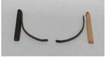
Once the height was good I glued the bent brass strip....1/64" x 1/16" brass strip to the wood stanchion (left side above). It's the same width so it will all look like the same piece if carefully sanded and painted and weathered.
