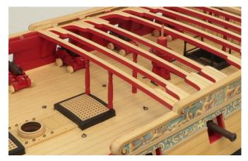
These two columns will need to be lined up perfectly with the Main jeer bits.....and gallows and chain pumps. The crank handle for the chain pumps will run through all of these elements and they won't be glued into position until after the chain pumps are made and everything is test fit together. That will come soon. So just position them like this without glue or set them aside.
