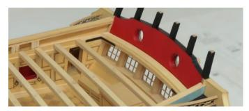
Before adding the iron brackets however, I added a strip of 1/8' x 1/32" cedar to deck clamp between both beams to clean it up and make the deck clamp flush with the paneling below it. Then I added the strap section on top of that....I am referring to span between the deck beams.
