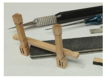
The jeer bitts were painted red and positioned beneath the Breast beam or that first qdeck beam. Nothing is glued in yet....these are just tests in preparation for completing the chain pumps. It rests right against the coaming behind it. The cross beam is on the aft side. But I will mention....
