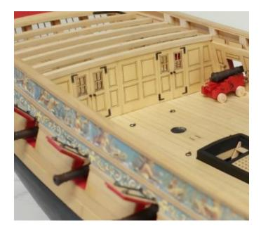
With this bulkhead completed, I can glue a couple cannon in permanently now and move forward to the work on the mast coats and then the next forward bulkhead. I will slowly work towards the waist in this fashion.....slowly adding the beams and knees as I finish making the fittings that will go under them.
