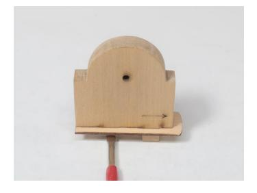
STEP 3 ...Glue the larger side panels onto the core. Sit the bottom edge of these side pieces right down on the base. Dont sand the char from the edges yet. Make sure the arrows are pointing in the right direction. They follow the arrow on the core. The important thing with this step is to line up the center hole for the crank shaft. That is crucial.
