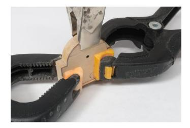
After both of those initial layers are in position you can sand the char from certain edges. Allow me to explain. The photo below shows the sides sanded FLUSH with the core and clean from char. But leave the rounded edges of the top and dont sand that at all. But the little edges on either side of the rounded top should be sanded flush with the top of the core. Note the back edge of the floor or base is now sanded as well as the back side is all flush with the core.
