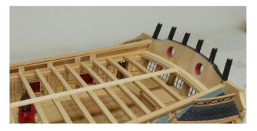
Lastly add the 3/64" thick top layer (the margin plank). See how it creates a rabbet or ledge for the deck planking. The last beam is actually a pretty good width and leaves a nice size ledge for the deck planking.
