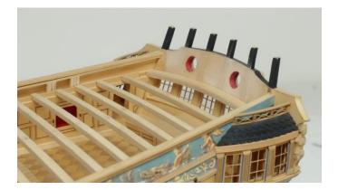
This beam has the same round up of the others but also conforms to the curvature of the transom. It's a tricky beam to make. The margin plank will sit on this leaving a rabbet along the front edge to seat the Q'deck planks into. It is laminated from two layers of laser cut cedar.
