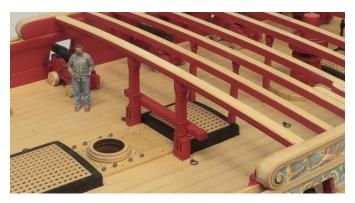
This is important, the Breast beam is actually wider than all of the other deck beams. Its 3/16" wide. In addition, you must scrape a
