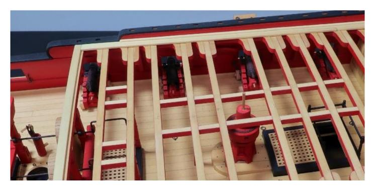
used a 3/16" x 3/64" strip for this. The overhang edge on both were rounded off. There is only a slight overhang along the breast beams with these planks which should leave you with a nice rabbet on the other side for your deck planking which we will start adding shortly. The rabbet was about 1/16" wide on the other side.
