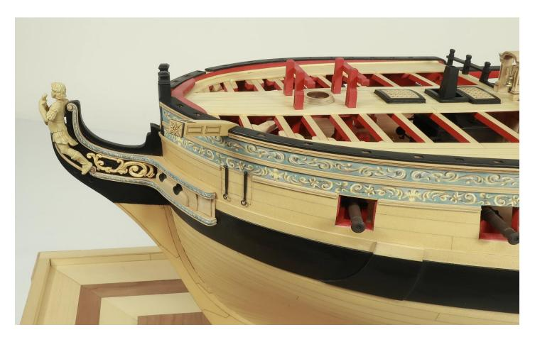
shown n models. The angle of the front of the cathead is important and before you glue the star onto it you should make sure its flat and shaped appropriately. Look at the laser cut sheet and I think you can better see the actual shape of the cathead on the side panels. I made sure I gave you guys an extra cathead just in case.
