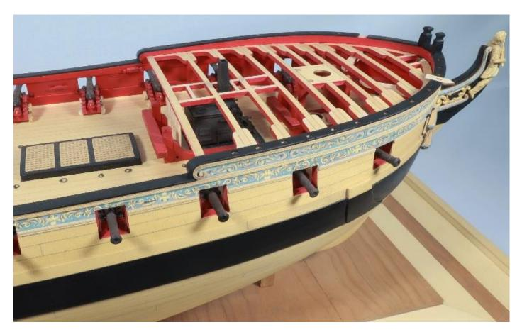
to widen the slot later and not so easy to make it smaller so be cautious here. Than the hance caps at the aft end of the fcastle were made as before. The two halves glued together so we have a nice wide piece. The hance caps were shaped and sanded for a snug fit. Then care was taken to eliminate any seams between it and the cap rail.
