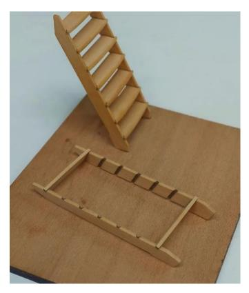
Finally I slid the remaining steps in position after applying a small drop of glue to each side. They slid right into place without much trouble. Once you do one or two it gets easier......carefully push them straight in and back.
