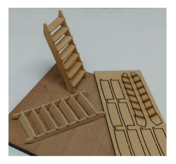
The top step is a bit deep which you will soon discover, so at this stage I used a sanding stick to sand it flush on the back side of the step. Then to finish it off I sanded the sides of the ladder to make those little "wings" on each step flush with the sides of the ladder. I hope that makes sense... as I left them a bit longer so they would need to be finish-sanded.
