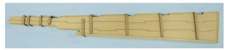
pintels. Then the outside surfaces were sanded thinner after the strips were glued all around the rudder head. I also sanded the sharp corners so they were softened up a bit. Take this time to mark the locations for the bolts along the straps with a sharp pencil. See the photo above.
