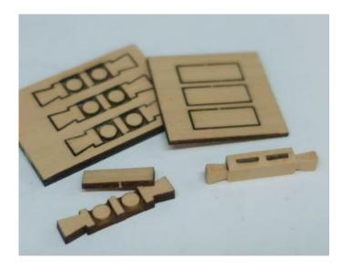
Basically the first thing you do is add the backing piece which will enclose the simulated sheaves. Those are laser etched as you can see above. The two "horns" (for lack of a better word) need to be shaped afterwards. These are the ends which need to be shaped like a typical timberhead on each side. I used a #11 blade to do this. Otherwise it would be flat ...you can see the front of the finished piece above. Then I lightly chamfered the edges...again like you would do with a timberhead.
