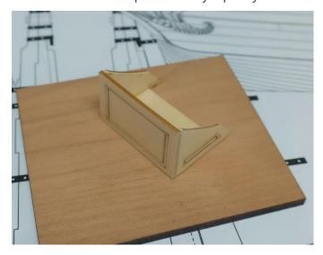
Then add the top. Keep in mind that the aft edge of the top is beveled so it fits snug against the curved counter planking. The top
