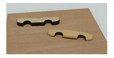
Then shape the forward side keeping it a consistent thickness. To finish it up round off the top edge as shown. IMPORTANT NOTE: Do not glue this in position. Just make sure it fits and looks good sitting on the cheeks. You don't want this glued on when you drill out the hawse holes. We will be doing that next. They would certainly get damaged.
