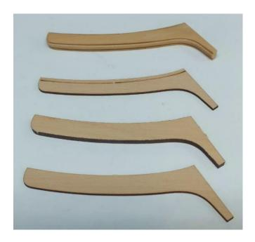
You should start shaping the middle layer first. Make sure it fits in position. Make sure it sits against the hull planking reasonably well and also against the stem. Everyone's model will be different because these are pretty
