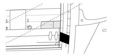
Its a little tricky but the reason why I wanted to mention it is because it's a detail often overlooked. In fact I am sad to say that I indeed also forgot to adjust my angle upward when drilling that first hawse hole. Now it wasn't a catastrophe by any means....but it does make me feel stupid. Of all people to forget to adjust the angle even after I went through the trouble of showing it on the plans....
