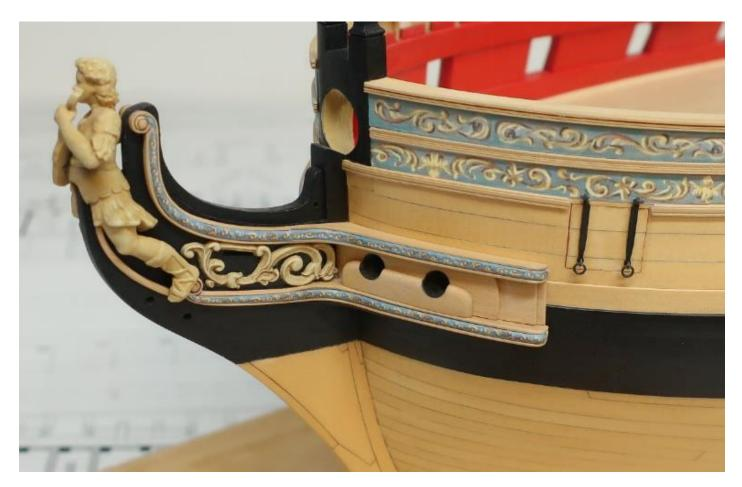
Here is a shot of the cheeks and hair brackets on the port side. Let me detail how they are made next. It's quite a long process even with most parts laser cut for you.
