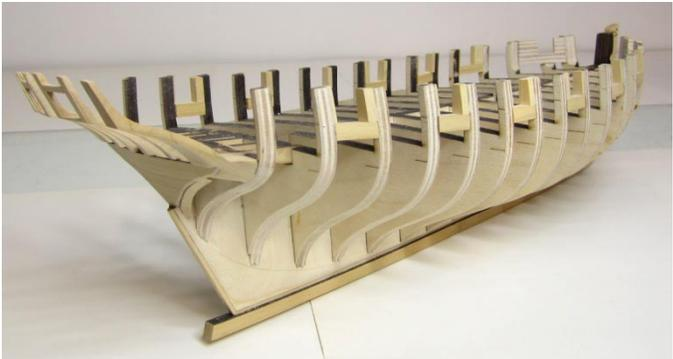
Finish this step by placing two filler pieces behind this square tuck piece. You will be gluing the plank ends here and need more surface than the 1/32" thick sheet can give you. You can use any scrap you have. I used pieces that were 1/4" thick. Once glued to the back side of the square tuck, they were faired as shown in preparation to receive the planking. Another view of the finished stern is seen below. This completes work on the skeleton of the model and we can now start planking the hull.
