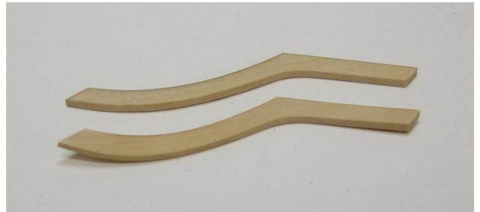
When gluing them on the hull, it is important to note that the fashion pieces will stand proud of the transom planking. They will be flush with the edge of the counter but along the transom, they will stick out about 1/32". It is hard to see this in the photo below but this overhang is important because the cap rail for the transom and the molding below the gunports will not look as nice without this small detail. Note how I left the fashion pieces a bit long as well. You should do
