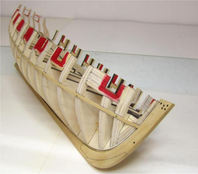
this just like you did when getting the smooth run for the port sills. Make sure you place the batten on both sides of the hull and check it carefully for dips and bends until you are satisfied with the run of the planking. It may not line up perfectly with the reference marks at this point and you will have to make tiny adjustments to get a smooth run.
