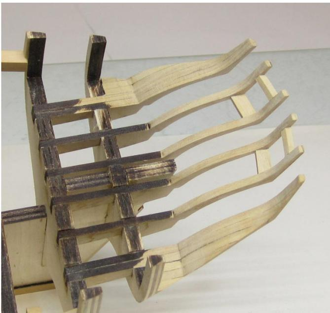
In this second photo, you can see how thin they must become. I used a small sanding drum in my rotary tool to carefully remove most of the excess thickness and then finished it off with some sanding sticks.
