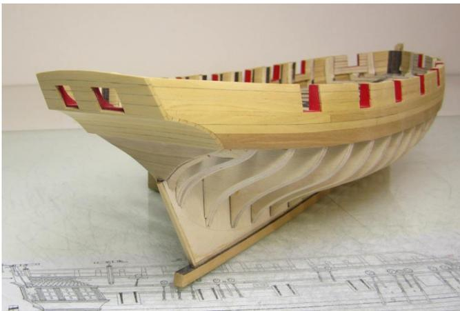
Here are a few inboard views after the stern planking was completed.
