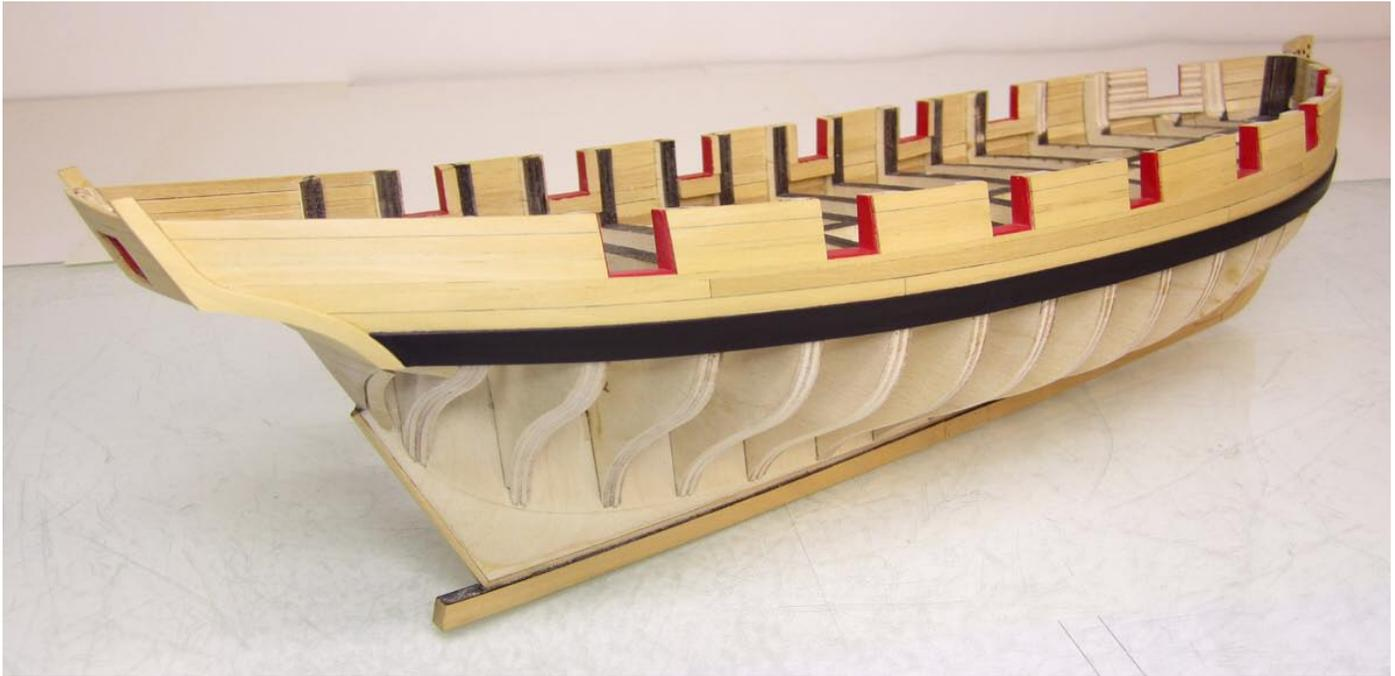
the same as leaving a bit of wiggle room above the sheer will make it easier to add the boom rests on top later in the project.
