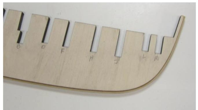
It is now time to add the rabbet strip to the bottom edge of the FK. The rabbet strip is a 1/8" x 1/16" strip of boxwood. It is glued down the center of the false keel's edge. This should leave 1/16" on both sides of the rabbet strip. As shown in that
