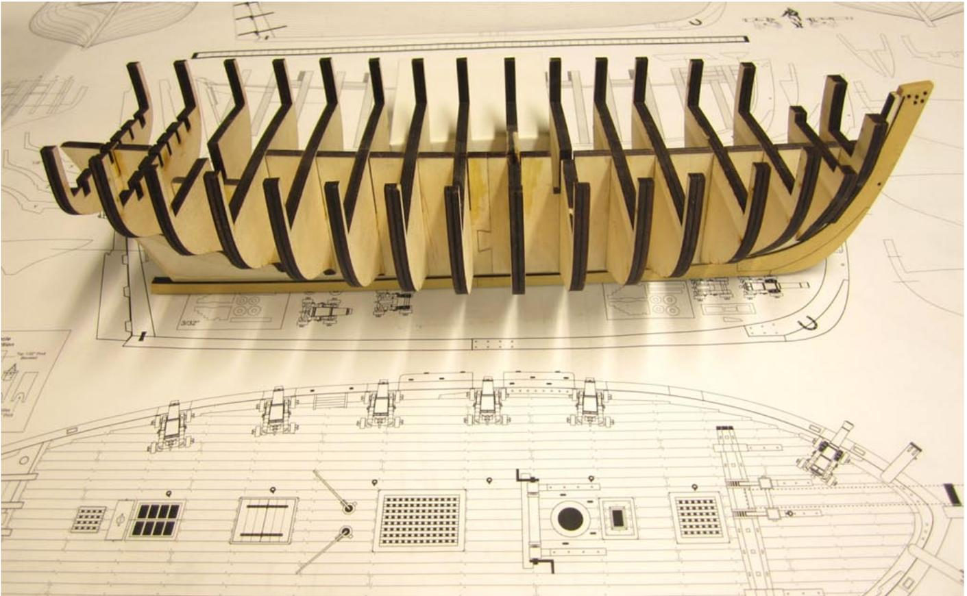
positions if they were placed in the opposite directions. On the prototype they were drawn on both sides but that is misleading and should be ignored if seen in any of the photos...so be careful when aligning yours.
