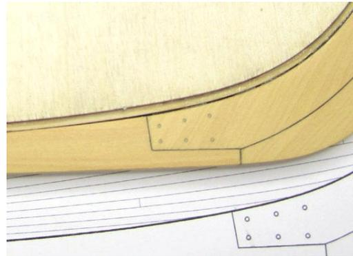
Next, the stem was glued to the rabbet strip. Be careful to line it up and center it along the rabbet strip. You should have a nice rabbet formed afterwards with equal space on both sides after it is centered properly.
