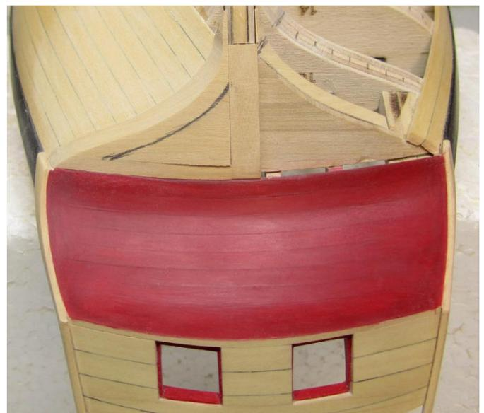
With this piece temporarily glued in place, fair its edge to the hull planking. You can see this has been completed in that same photo on the previous page. With its true shape now defined, draw another reference line along the edge so you have the last timber measured at  $1/8$ " wide.
