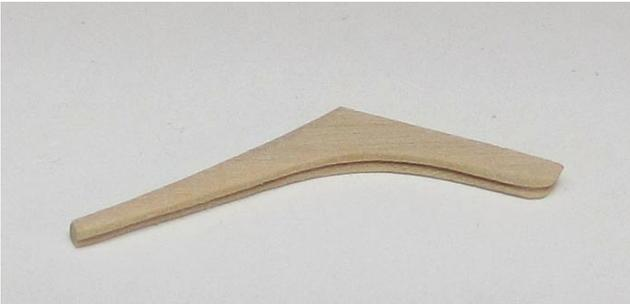
I found it was easier to make a template out of card stock first. Then use the template to cut a slightly over-sized blank. After sanding it so it fits snug against the hull and stem, I scraped the profile to match the beaded molding. The edge that fits along the hull and stem needs to be beveled because of the complex angles involved.
