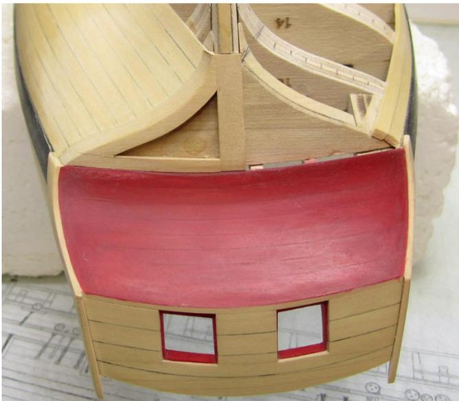
All that remains is to plank inside the frame. The planking is vertical and I started against the middle strip. The planking is  $1/8$ " thick by  $3/16$ " wide.
