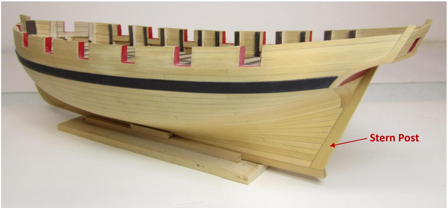
When the second belt has been completed on both sides of the hull along with the square tuck, you can add the stern post. The shape of the stern post can be found on sheet one of the plans. I used a soft pencil to darken the inside edge. You can see the darkened seam between the stern post and the planking above. Carefully shape and adjust the inside edge so it fits snug against the planking and square tuck with no gaps between the two.
