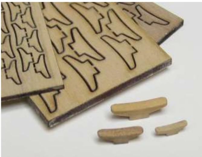
They were sanded to remove the laser char and shaped a bit. Then they were glued into position. A small length of wire was used to pin them into pre-drilled holes. I just went ahead and added all of the cleats found at the stern and along the bulwarks.
