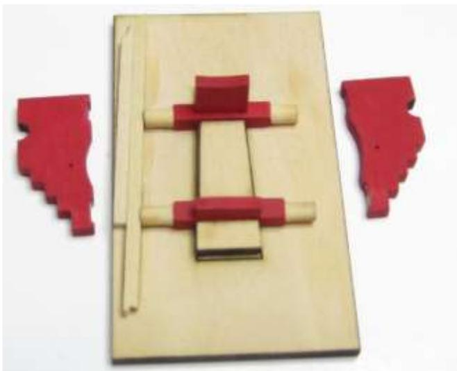
To begin, I removed all of the laser char from each piece using a sanding stick, emery board and needle file. Then the ends of the axles were rounded off for the trucks (wheels). Next I decided
