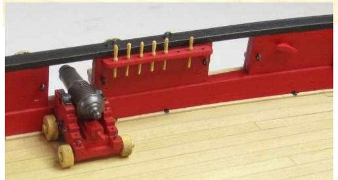
These boxwood belaying pins will not be as strong as the brass versions you can buy. But I am a light-handed rigger!! I won't pull the rigging so tight that they would be in danger of breaking.
