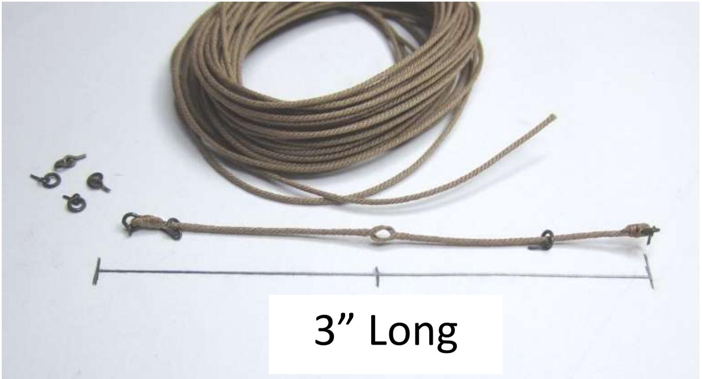
The eyebolts with split rings were made in advance. You will need four of these to make each breech rope. Seize the first ring the end of the breech rope. I used sewing thread for the seizing.
