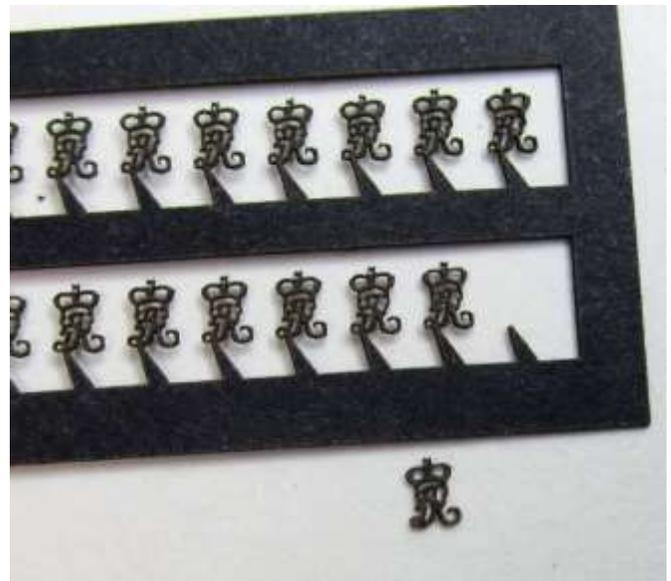
make sure you wash the m thoroughly to remove any residue and oils that may affect the paint adhesion.
