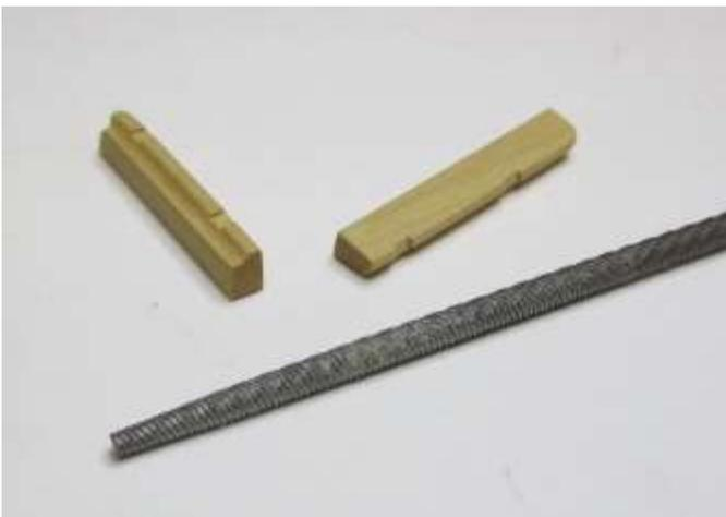
When viewed from the side they gradually get thinner but a little bit. The bottom is beveled or angled so the outboard edge is just 1/8" thick. Maybe a hair thicker. But it is not as thick as the edge that fits against the hull.
