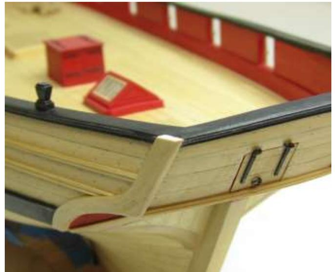
I cut an over-sized version of the boom crutch out of boxwood. I used a  $\frac{1}{4}$ " thick piece to cut it from but really should have gone a bit thicker. I made sure there was a lot of extra meat on it so I could slowly sand and file it to shape, creating the four proper angles needed. The tail or the stem of the blank crutch was purposely made wider and longer to start.
