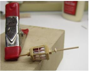
added at this time. Again, these are really tiny pieces and should be shaped on the end of a stick to clean them up. Part "D" is placed on
