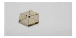
After a test fit to ensure that the three wedges (part # 2) fit, glue them into position with some white glue or carpenter's glue. It is best to do this on a flat surface. Sand the edges to remove most of the laser char and get a nice tight fit.
