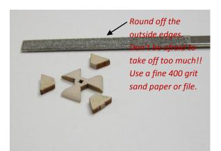
Remove part #1 from the laser cut basswood sheet. This piece looks like a "Y" shaped piece and will become the basis for creating the hexagonal bottom of the lantern. It is sometimes difficult to take a hexagon and sand it to shape consistently without altering the neat, clean hexagonal facets. To overcome this, you will be shaping three facets at a time.
