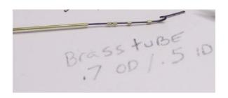
2. Cut the brass tubing into small sections. They should be the same 1mm width as the hinge straps. DON'T USE CUTTERS!!! The only way to cut this micro tubing without crushing it is shown in the photo above. Insert a length of 28 gauge wire into the tube. Roll a sharp Xacto blade over the tube until a small 1mm section is parted off. If you bend the end of the wire they will all collect nicely on it rather than bounce all over your workspace.
