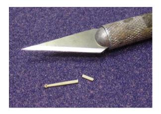
1. Remove a laser cut hinge strap from the sheet. Cut it to the length you will need to fit your port lid. A sharp Xacto blade works well.
