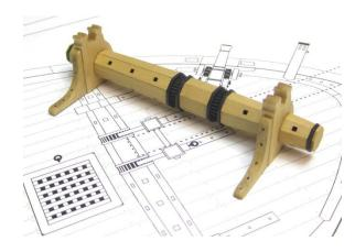
Final Assembly - Slide all of the segments onto a strip. Sandwich them together tightly as a dry fit test. Remember to place them in the correct order and orient the holes properly on
