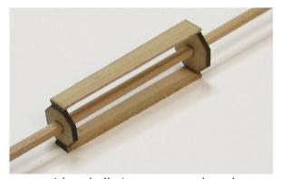
start with a shell piece on to and on the bottom first as shown below. This will stabilize the segment and make it easier to add the remaining outer shell pieces. Carefully line them up on each face of the octagonal pieces or you may have some gaps when you try to insert the final piece.
