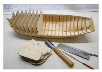
Below is a photo of a frame center on another project being removed. In this example a file is being used to cut the small tabs.
