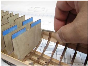
Then the frame center is gently bent back so it snaps free at the bottom and can be removed.
