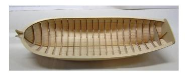
Above you can see the 1/16" thick laser cut caprail glued into position. It is made of 4 laser cut pieces. They are made very over-sized and we will thin them down considerably later. But you want a decent overhang inboard and outboard to begin with.
