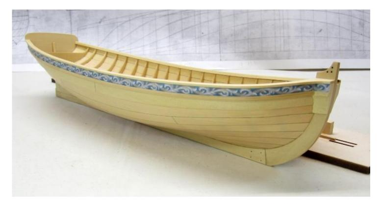
The friezes are provided already shaped like a prespiled plank. They should conform to the hull well enough. Try and hide the seam between the two halves mid ship as best you can and match the pattern like you would when you hang wallpaper. Then cut off any excess length at the stern flush with the transom. There is also a small length of frieze on your sheet that should be added to the bolsters at the bow. Cut of any excess flush with the front edge of the bolster.
