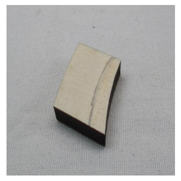
I used sand paper and files to create the bevel. I stopped and tested how it fit dozens of times as I continuously tweaked it. The photo below shows that I almost have a good fit. There was plenty of meat on the blanks so you can sand and reshape quite a bit. So just keep going until it fits well against the planking.
