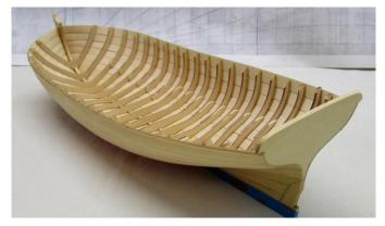
The next step will be fine tuning the sheer. Sand the tops of the frames down to the sheer and also sand the sheer so it has a good smooth run from bow to stern. You don't want any dips or high spots. These can be seen by viewing the hull headon and stern-on at various angles. Once satisfied we will add the caprail which is laser cut for you.
