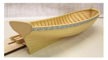
Use the bottom edge of the frieze to align the molding strip below it. The molding strip is 1/8" x 3/64" and it is scraped to a simple profile. You were provided with boxwood strips for this in the kit.
