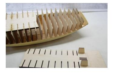
Turn the model over (actually right side up). Remove the tape holding both halves of the build board together. Then carefully and gently coax one half of the build board free. Don't rush this and slowly pry it off a little at a time working one side then the other. It will be tricky to get it started especially on a humid day. But once it starts wiggling free it will come off readily. Do the same with the other half.
