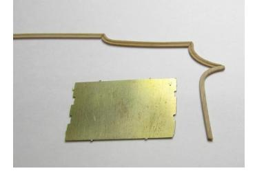
Adding the knee inboard at the bow was next up on the agenda. This is pretty straight forward. The knee will need to be curved to match the sheer at the bow. The top edge of the knee should sit flush with the top of the cap rail. Once painted, you don't want to be able to see any seam between the knee and the cap rail. This means you will have to bevel the edge of the knee also so you get a really tight seam between it and the cap rail.
