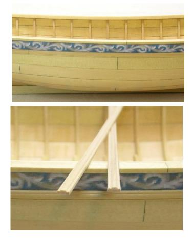
The last photo shows the profile I chose for the fancy molding below the frieze. This can be created in the usual way. The profile was filed into a thin piece of brass or you can use a razor blade. Then the scraper was lightly run over the boxwood strip until it created the profile you see in that photo. You can see a similar scraper below which was used on another project to create the fancy molding profile. This was done the same way.
