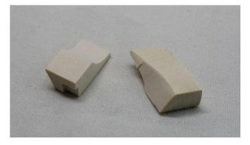
Note how you will need to make a matching pair of these. The only difference is that a small notch needs to be carved out of the top of the one for the roller. You can see that in the photo above. It adds more room for the roller. It's shown on the left.
