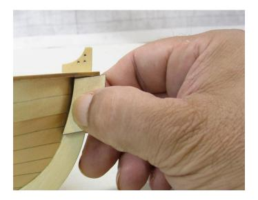
I have *guestimated* the amount of bevel required before I started, marking it in pencil. Note how there is more of a bevel towards the bottom of the bolster. You should do the same as it is good to have some sort of guide even though you are just guessing at this point.
