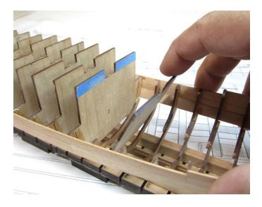
And finally, here are some pictures of the longboat model after removing all of the frame centers.
