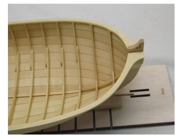
In the photo above you can see how the cap rail was finally sanded to shape. Note how the inboard edge against the stem is flush. This is important as you will be adding a knee against this to further shape the cap rail behind the stem.
