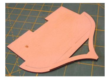
Test it in the corresponding slot of the build board. BUT also test the bottom to see how it fits in the keel. The notches in the keel were also made a bit small so they would be a snug fit. But if the frame doesn't fit into the keel notches, file it a bit until you get a nice fit. Perform this exercise for each and every frame to check their fit into the build board slots and keel notches as you finish them.
