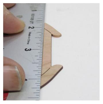
Then take the floor and slide it up against the metal straight edge. You will see that it fits nicely but be careful to position it properly from side to side. Do a test fit first before applying any glue. Only apply the glue to the bottom portion of each top timber. Be careful to not get any glue in the cut line between the top timber and the frame center. This will make it more difficult to remove later on.
