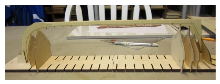
Above you can see what the keel assembly looks like after being tested on top of the five single part frames. Note how the two halves of the build board are not glued together. You should never glue the two halves together. Keep them separate for the time being. You can remove the keel assembly while you are building the two part frames next.
