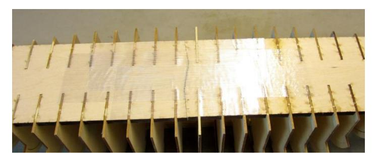
Here is the model after it was completely faired. You can use the laser char on the edge of each frame as a guide as you continue fairing as well.....onto planking in the next part of the project.
