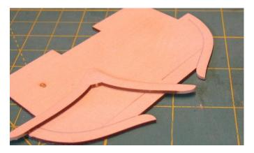
The remaining frames are made by gluing the two pieces together. I recommend that you only work on one frame at a time. The top timbers are also numbered but once you remove the floors (bottom piece) from the laser cut sheet, there is no identifying number or letter. So only remove the two pieces for one frame at a time to avoid mixing up the floors.
