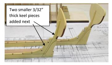
The three 5/32" keel parts on the simplified version all glued up. The four 3/32" notched parts are shown and are ready to be glued into place next.
