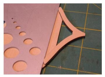
You only need a little bit of glue. I recommend that you use titebond or some other yellow glue. Don't use CA Glue. It sets too quickly and you want to have time to slide the floor one way or the other so it is positioned correctly. The finished assembly is shown below.
