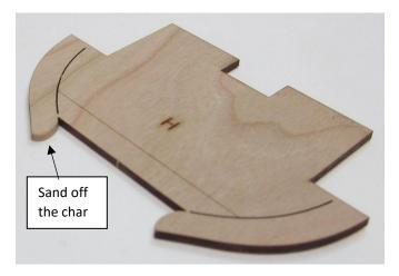
The top timbers are held in place by the tiniest little tabs. Be very careful with these because you don't want to separate the top timbers from the frame centers. Carefully remove the laser char from the tips of each top timber only. Once again, don't worry about the rest of the frame edges.
