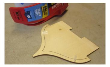
In addition to the tape, you can add a small length of cedar strip across the top of each frame at its most vulnerable point. You can see them below. Use small lengths of 1/16" x 1/32" strips. This will be hidden once planking is finished inboard and outboard. It really does help stabilize the frames while you plank and fair the hull. I only added them on the one piece frames but you can add them to one side of all the frames if you like.
