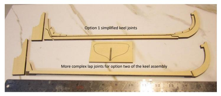
You can see that the three parts for the more complex keel assembly (5/32" thick parts) shown on the bottom of that photo are joined using lap joints. I have not removed any laser char from the edges of these pieces yet. It is better to leave that intact until after "carving" and completing the lap joints. In the photo below you can see two of each part.
