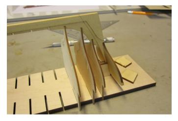
The two transom blocks in the slots can be moved forward or aft so you can get a good fit against the transom. Remember that they are not glued in. The slots for them are longer than needed so they can be adjusted to best advantage. But once in a good position, you can add the two smaller brace blocks.
