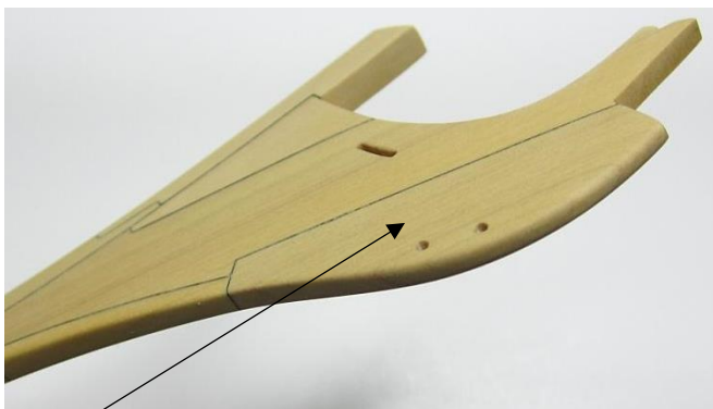
Bobstay piece tapered toward the forward edge ...you can even taper the stem a little below this point if you wanted.
