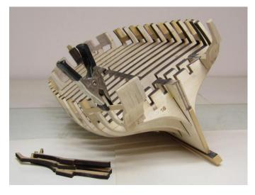
might be able to see that the starboard side has been faired already. To do this, I ran a longish strip of wood down the side of the hull. You can see it clamped to the bulkhead above. There is no need to clamp it. I just need to do so in order to show you the strip in place. As I ran the strip down the hull the aft end was traced on the inside of the stern frames. This created a close representation of what the faired shape of those stern frames would look like. See the image below.
