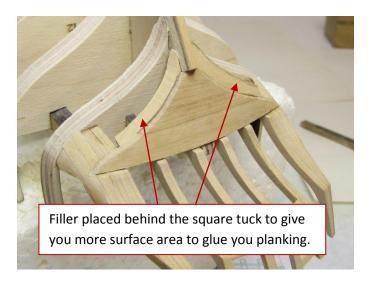
Finish this step by placing two filer pieces behind this square tuck piece. You will be gluing the plank ends here and need more surface than the 1/32" thick sheet can give you. You can use any scrap you have. I used pieces that were ¼" thick. Once glued to the back side of the square tuck, they were faired as shown in preparation to receive the planking. Another view of the finished stern is seen below. This completes work on the skeleton of the model and we can now start planking the hull.
