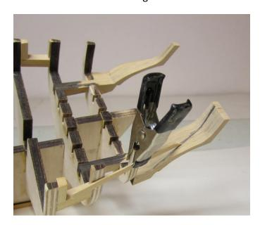
With this reference line drawn as shown, I was able to quickly remove most of the excess wood with a sanding drum on my rotary tool. When I got close to the line I stopped and finished fairing the outboard edge of the stern frames by hand.
