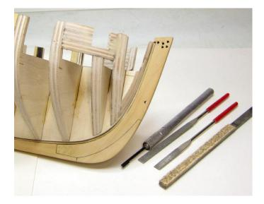
All that remains is to cut the port using whatever tool you feel most comfortable using. I prefer using a scroll saw blade. I snip it into smaller lengths and place it into the handle of a hobby knife as shown above. Its slow work but does the trick. Then I used various sanding sticks and files to make it look sharp and pretty.
