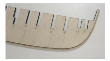
It is now time to add the rabbet strip to the bottom edge of the FK. The rabbet strip is a  $1/8" \times 1/16$ strip of boxwood. It is glued down the center of the false keel's edge. This should leave 1/16" on both sides of the rabbet strip. As shown in that first photo, the rabbet strip is also extended up the back edge of the FK to where the small notch is located.
