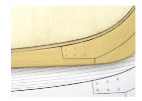
Next, the stem was glued to the rabbet strip. Be careful to line it up and center it along the rabbet strip. You should have a nice rabbet formed afterwards with equal space on both sides after it is centered properly.
