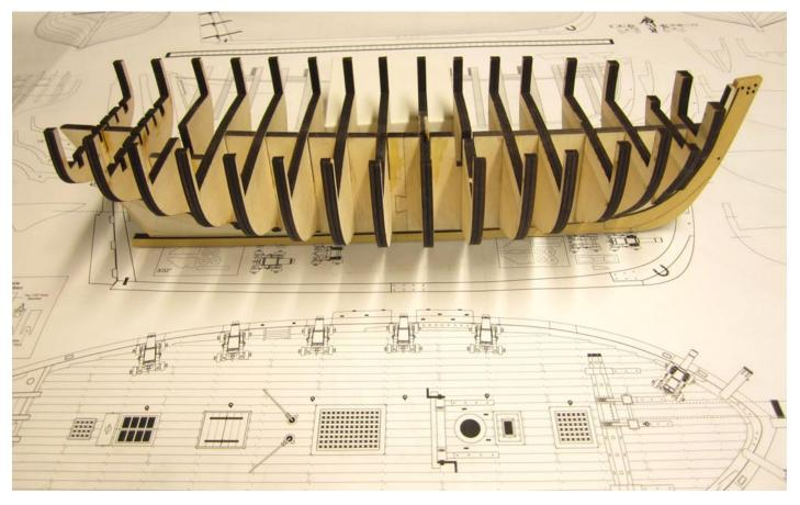
positions if they were placed in the opposite directions. On the prototype they were drawn on both sides but that is misleading and should be ignored if seen in any of the photos...so be careful when aligning yours.
