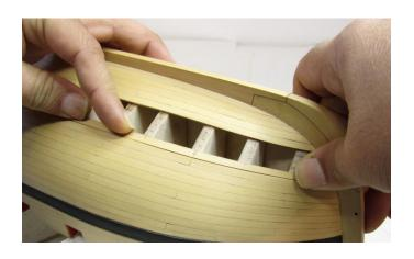
9. I must also point out that you will have to bevel the edge that butts against the strake already on the hull. This will make it so you get a nice tight fit against the existing plank. Then I run a number 4b pencil along the edge to simulate the tarred seam. Remember to cut the plank to the proper scale
