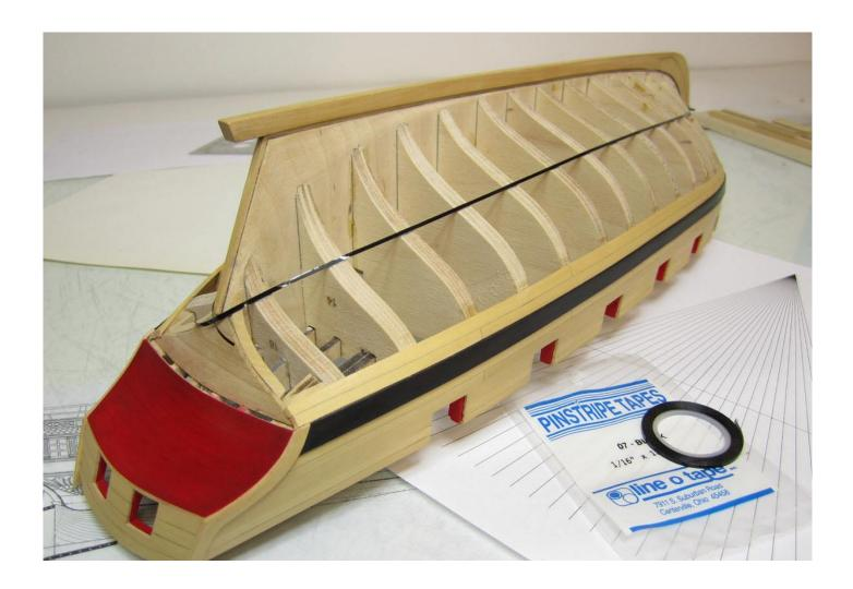
The pinstripe tape is self adhesive so once you have the locations at the bow and stern, you should adjust it at every bulkhead edge until you have a smooth run. Take your time examining the run of your tape as it will become the run of your planks. Make tiny adjustments until its smooth and true when viewing it from every angle. I do this on both sides of the hull to ensure it is the same.
