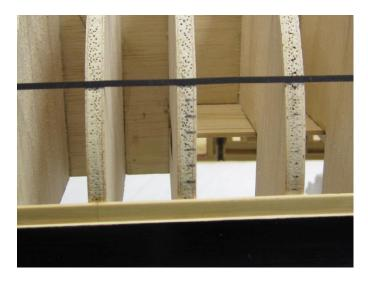
What you will find is that the plank segments will get narrower at the bow where they must be tapered. At the stern along the square tuck, you will see that the planks remain pretty much 3/16" wide all across the hull. No tapering or widening is required in this belt. I did not have to adjust any of the planks at all in this first belt except for the first 4 or 5 bulkheads at the bow. That is where some tapering is required.
