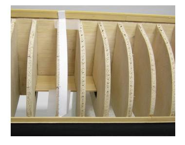
I find using a planking fan another good technique for quickly dividing a tick strip equally into segments of any width. I have provided one for you on the next page. Just lay the strip on top of the planking fan which has equally spaced radiating lines. Moving the strip evenly up and down will give you perfectly spaced segments. I have already marked a center line where the segments are 3/16" wide. Just lay your tick strip across the
