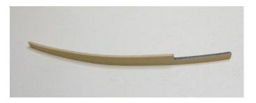
The shape of the drop plank is unusual. Rather than try to create it from wood right away, I used some stiff card stock to find its shape first.
