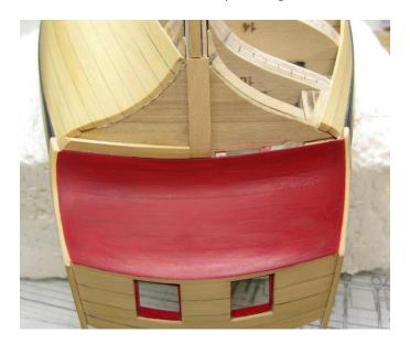
The final piece of square tuck framing is a bit tricky. Hold a piece of 1/8" thick sheet against the square tuck. You need to first create the same curve so it sits snug against the timber you just finished. It also needs to sit flush against the center strip, see below.
