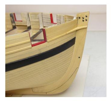
Its best to fit the small "ear" that crosses over onto the stem first. Then add the small length of molding behind it. The tricky part will be matching the beaded profile along the edge of the ear. This was scraped into the edge of the "ear" using the same scraper. Pictured below is an image of the ear after it was shaped and scraped.
