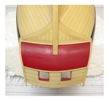
To complete this chapter, I added the keel plates and horse shoe Plates to the keel as shown on the plans. Normally these are made from thin brass sheet and blackened. Instead I used the laser cut parts available from siren Ship Model Company.
