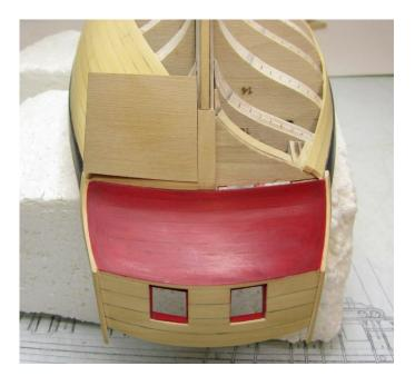
Then take a pencil and trace the shape of the hull on the other side as it sits against the hull. You can see my reference line below after removing the piece.
