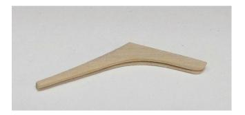
I found it was easier to make a template out of card stock first. Then use the template to cut a slightly over-sized blank. After sanding it so it fits snug against the hull and stem, I scraped the profile to match the beaded molding. The edge that fits along the hull and stem needs to be beveled because of the complex angles involved.
