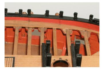
Note how the scarphed planks sit against the waterway rather than being cut into it as shown on the plans. The same will be done at the stern on the Cheerful model. To do this, we must line-off the deck in much the same way that we did for the external hull planking.
