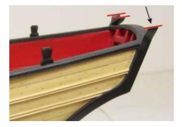
See the angles established in red (above) so the crutches match the sheer or are at least level rather than slanting upwards. This is important and the bottom of the crutch....inside the crutch... should also be addressed and angled downward slightly or at least leveled off if need be. Think about how the boom would REST in each crutch when establishing the angle inside the crutch.
