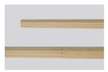
Then choose whatever method you feel most comfortable with to shape the outboard end into a neat octagon. I prefer to just use a #11 blade and slice off the heavy stuff just a bit outside of the lines. Then I use a sanding stick to finish it off.
