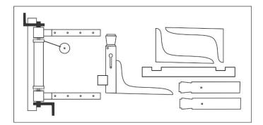
The only remaining parts of the winch were its handles. There are many ways to make these. I used a small thin piece of boxwood with a hole drilled through its end. Then a piece of 24 gauge wire was inserted into this hole to simulate the crank handle. To finish it off, a small (very tiny) length of micro tubing was glued onto the end of the crank handle wire. This gave it more detail and finished it off nicely.
