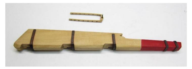
edges. The rudder is tapered as it works its way aft. The profile for this tapering is shown on the plans. The taper also exists as the rudder proceeds down to the bottom edge. The photos also show the shape.
