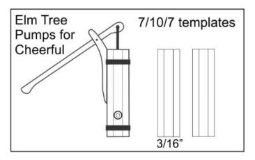
1. Transfer the 7/10/7 template lines to each side of the 3/16" square pump tubes. Carefully file the tube to an Octagon using the lines as a guide. Drill and bore out the top of the tube to a depth of about 3/8". Carefully use a bit that will leave the pump tube walls not too heavy.
