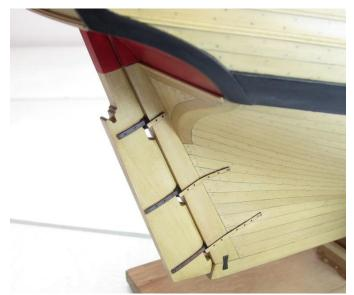
The rudder was hung as a test so I could mark the area of the rudder head that was to be painted red. I also used some weathering powder on those pintles and gudgeons so they would more realistically look like simulated metal. The same thin material was used to simulate the two metal band around the rudder head.
