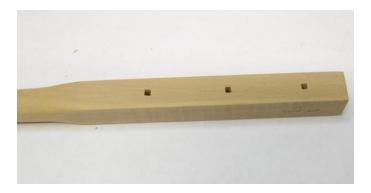
Step six – Test the bowsprit in the hole you made for it through the bulwarks. You should be able to slide it all the way up from the inside. But be aware of all of those deck fitting you worked so hard on. You don't want to break any of them.
