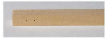
Step two – prepare the outboard end of the bowsprit for rounding. To do this, use the 7-10-7 ratio just like we did when making the octagon pump tubes. The outboard end of the bowsprit will be planed, or filed to an octagon before you can make it round. So mark each side of the stick with lines using the 7-10-7 ratios. See below.
