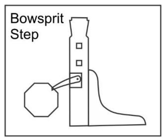
Assemble the three layers for the uprights. Then use a needle file and sharp chisels to finish shaping the top of both of them. They will look like the timberheads along the cap rail and the top of the winch uprights when you are done.
