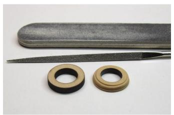
Many contemporary models have stylized mast coats with a fancy profile. A small washer of 1/8" thick boxwood was made. Now if you are fortunate enough to have a lathe or even a vertical milling machine, there would be countless ways that you could make the mast coat. But if by chance you do not, the mast coat can be shaped by hand by careful use of needle files, emery boards and sanding sticks. This is the method I chose to use and the photo above shows the results.
