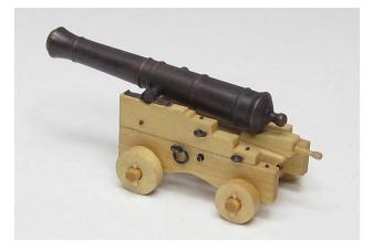
prevented them from twisting. See the photos for details. Don't forget to add the eye bolt on the back of the rear axle which can be easily overlooked. The larger ring for the breech line was made by wrapping the 28 gauge black wire around a drill bit several times. Then each ring was parted off with a flush cutter or wire cutter.
