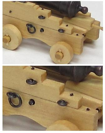
holding the two sections together. It's a small detail but you might want to give it a try. The line was etched with a sharp awl. Use a metal straight edge as a guide.
