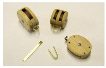
open. Glue them into position well so the strap doesn't come loose when rigging the block.
