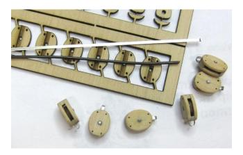
**STEP 1** – Separate the three layers of frets and arrange them so they are close by so you can glue them together. Set the wire and brass strips aside for now. See below
