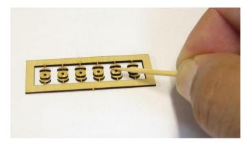
**STEP 3** – Add one outer layer before your glue dries. Line it up carefully. Make sure you use the outside of the fret to help you properly align each layer. It is very important.....VERY IMPORTANT...to make sure the laser etched slot for the brass strip faces toward the inside of the block. This is especially true for double blocks. The
