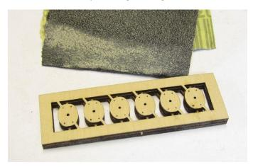
**STEP 5 - Carefully** remove the six blocks from the fret with a sharp #11 blade or even a pair of flush cutters. Cut each block free close to the frame of the assembly
