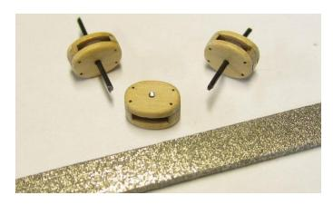
**Step 9** – Cut tiny lengths of the brass strip. For the smaller blocks Nickel strips are used. They blacken up nicely or can be left bright. They don't need to be very long at all. Then bend them into a "U" shape. Insert this into the etched slots which should be still open on the top or bottom of the block. It doesn't matter which end. But look for the side of the block with the open sheave hole first. Then you wont have to drill out the sheave holes for your rope later. One side is already
