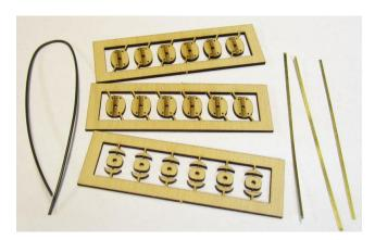
**STEP 2** – Use a toothpick to place a drop of glue on each part of the center layer. Make sure you get ample glue (medium CA) in the sheave and the top and bottom areas.
