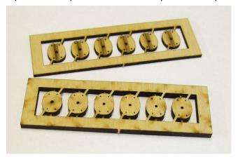
rope to slide through the block. Make sure that the open end is facing the same way on double blocks to avoid having to drill them out afterwards.
