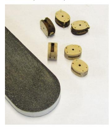
**STEP 7** – Place the blocks in your block tumbler and run it for just a 30 seconds on the highest speed. I am using the Model Shipways Blockbuster. It gets plenty of use in the shop as you can see below. The worse thing that you can do is over tumble these. Check them frequently to ensure they are tumbled nicely to just
